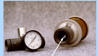
Sampling Equipment Opened to show Orifice Plate
