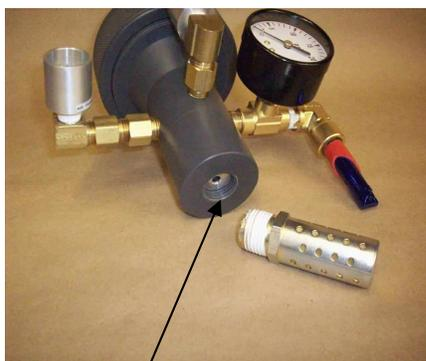
Orifice Plate with Noise Muffler Removed
