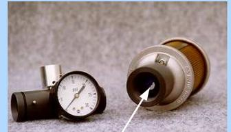
Sampling Equipment Opened to show Orifice Plate
