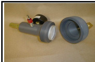
Both Halves of PVC Filter Holder Before Final Assembly
