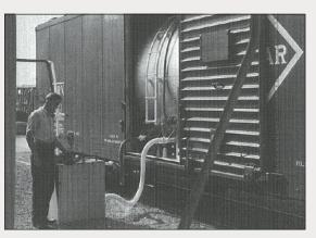
1930s Liquid Oxygen Railroad Tanker (Courtesy of: Union Carbide Corporation)
