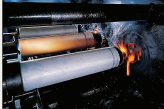
Aluminum Cylinder Neck Formation (Courtesy of: Luxfer Gas Cylinders USA)
