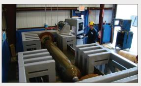
Ultrasonic Cylinder Testing (Courtesy of: FIBA Technologies, Inc.)
