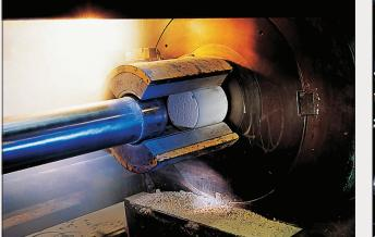
Aluminum Cylinder Extrusion (Courtesy of: Luxfer Gas Cylinders USA)
