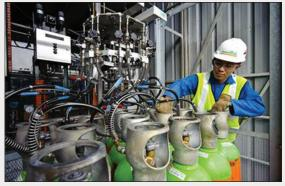
Packaged Gases Cylinder Fill Station, Malaysia (Courtesy of: Air Products and Chemicals, Inc.)
