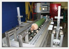
Ultrasonic Cylinder Testing Station (Courtesy of: FIBA Technologies, Inc.)
