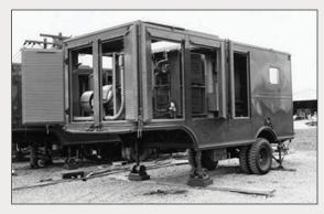
1955 Mobile Oxygen and Nitrogen Semi-Trailer (Courtesy of: Air Products and Chemicals, Inc.)
