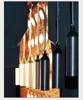
Aluminum Cylinder Painting (Courtesy of: Luxfer Gas Cylinders USA)
