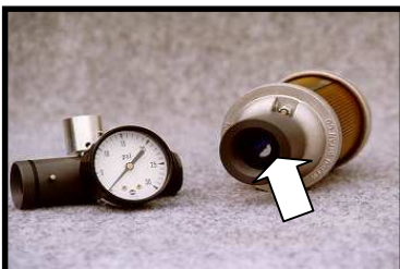
Flow Section opened to show orifice plate
